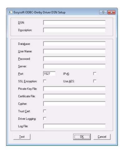
Figure 5: The Easysoft ODBC-Derby Driver DSN Setup dialog box
